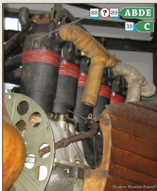
Benz Bz.IIIa 29031 fitted into Roland D.VIb 2225/18 in the Krakow Museum in Poland. Note the red bands painted around each cylinder indicating they contain over compressed cylinders.
