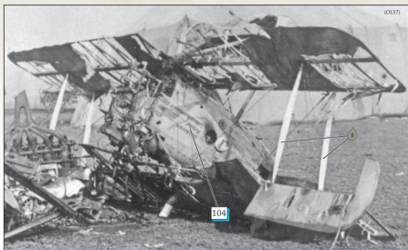
This unidentified late production Roland D.VIb has been partially stripped of its fabric and destroyed by fire.
