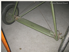
Undercarriage detail from Roland D.VIb 2225/18 showing the grey-green colour of the struts and various metal fuselage fittings. Note how the rigging enters the fuselage.
