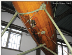
Undercarriage detail from Roland D.VIb 2225/18 showing the grey-green colour of the struts and various metal fuselage fittings. Note how the rigging enters the fuselage.
