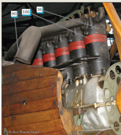
Benz Bz.IIIa 29031 fitted into Roland D.VIb 2225/18 in the Krakow Museum in Poland. Note the red bands painted around each cylinder indicating they contain over compressed cylinders.
