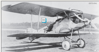
Roland D.VIb 7502/18 photographed during an intermediate stage of the camouflage experiment. Note how the 'dull black green' applied to the spine of the fuselage does not yet reach down to the top of the '75' in this photo. The propeller, struts, wheels, side of the fuselage in the shadow of the top wing, undersides of the wings, tailplane and bottom of the fuselage were aluminium. This was not painted on, it was covered with aluminium 'plating' (foil?) and 'aluminium powder dusted or burnished on'. The result is a highly reflective finish which appears both light and dark in this photo depending on what the surface is reflecting. Note the playing card 31 stuck inside the 'V' which had been removed by the time the hand tinted photos above were taken.
