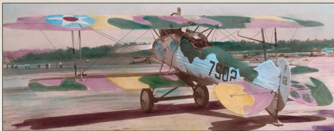
Roland D.VIb 7502/18 photographed during an intermediate stage of the camouflage experiment. Note how the 'dull black green' applied to the spine of the fuselage does not yet reach down to the top of the '75' in this photo. The propeller, struts, wheels, side of the fuselage in the shadow of the top wing, undersides of the wings, tailplane and bottom of the fuselage were aluminium. This was not painted on, it was covered with aluminium 'plating' (foil?) and 'aluminium powder dusted or burnished on'. The result is a highly reflective finish which appears both light and dark in this photo depending on what the surface is reflecting. Note the playing card 31 stuck inside the 'V' which had been removed by the time the hand tinted photos above were taken.
