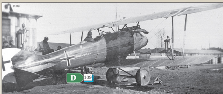
Late production Roland D.VIb 6142/18 in a similar camouflage finish to D photographed after the Armistice.
